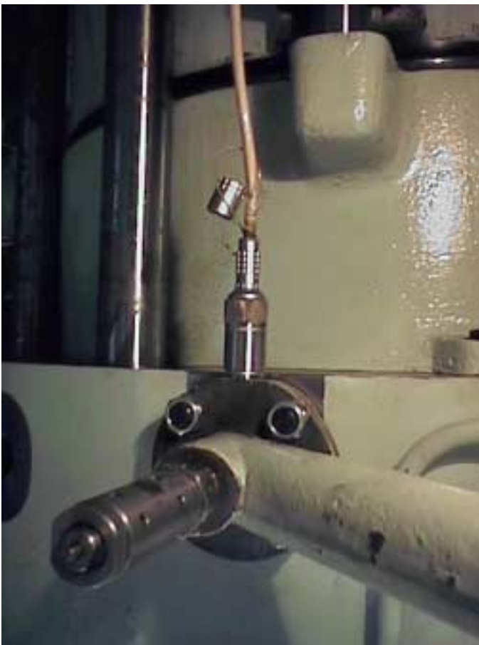
Fig.10: Sensor installation on a 2-stroke engine (Indicator flange)
