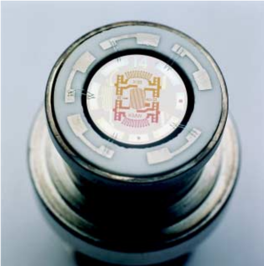
Fig.5: Thin film structures of a bonded measuring cell.
